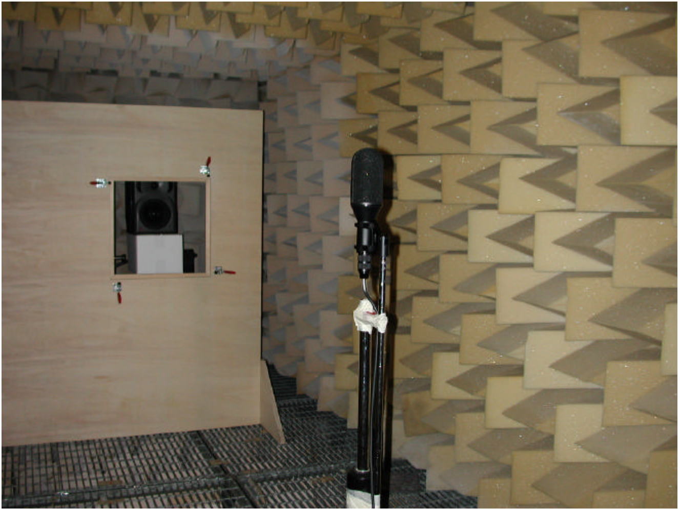
Fig. 1 – The Soundfield MK-V and the loudspeaker, in the WX and WY mounting mode.
