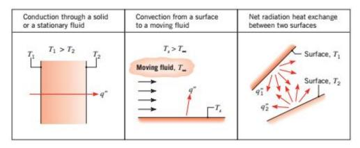
Figure 1. Conduction, convection, and radiation heat transfer modes (1).
