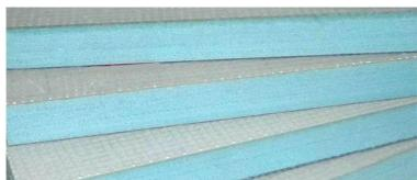
Figure 11. Extruded Polystyrene (XPS)
