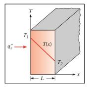
Figure 3. One-dimensional heat transfer by conduction (diffusion of energy)
