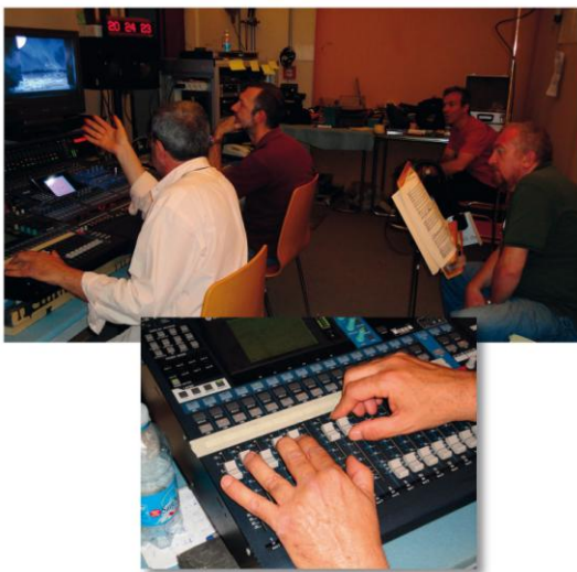
Figure 10 – Mixing of the 7 live signals live obtained through the 3D VMS system and the pit microphones.
