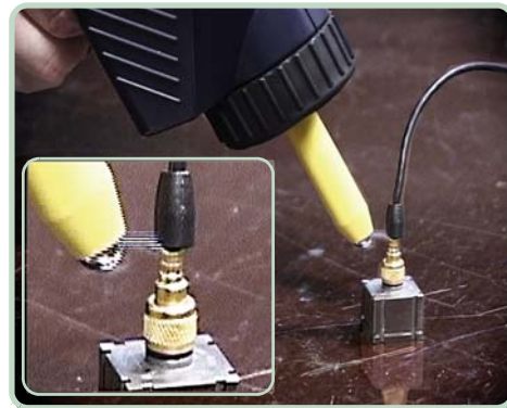
Electrostatic discharge immunity test as part of EMC testing
