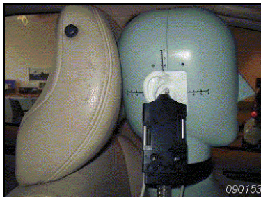
Fig. 21. Positioning the adaptor of mid-high-frequency sound source next to HATS right ear for reciprocal frequency response function measurements
