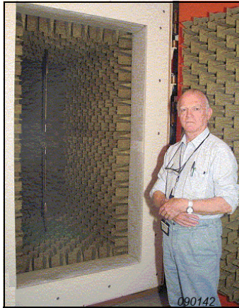
Fig. 8. The DFM/DPLA free-field calibration room. The microphone mounting bars were automatically moved between pre-selected microphone positions (In front: Knud Rasmussen)
