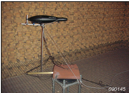
Fig. 1. Low-mid frequency sound source (without extension hose)
