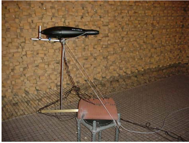
Figure 2: Picture showing the OmniSource™ with VV adaptor above a turntable
