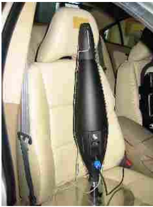
Figure 7: VV source in a Volvo60 passenger car
