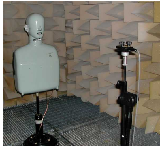
Fig. 3 – Brüel & Kjær mouth simulator type 4128 on the rotating table
