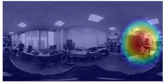
Figure 15. Colormap of two sources, coherence filtering with the static source
